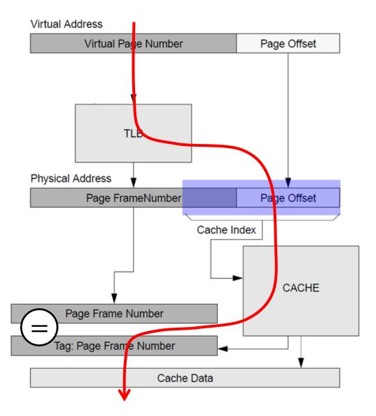
At hit, time to access memory includes TLB and cache accesses. The two can be pipelined.
