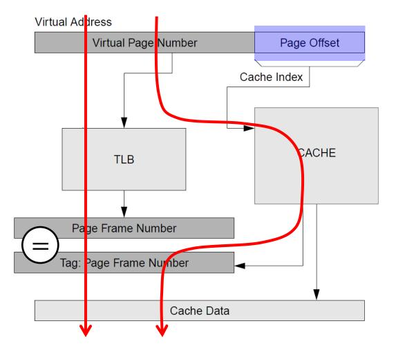
If cache index uses only page offset bits, TLB is eliminated from the critical path.
