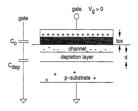
Inversion occurs when  $V_g$  is positive and > Vtn (for P material). A model for inversion in comprised of Cox A connecting from gateto-channel and Cdep connecting from channel-to-substrate.
