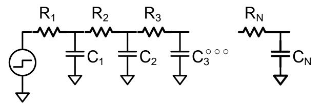
For a step input Vin, the delay at any node can be estimated with the Elmore delay equation  $\mathbf{t}_{Di} = \Sigma \mathbf{C}_i \Sigma \mathbf{R}_k$
