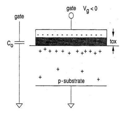
Accumulation occurs when Vg is negative (for P material). Holes are induced under the oxide. Cgate = CoxA where Cox =  $\varepsilon$ SiO2 $\varepsilon$ O/tox
