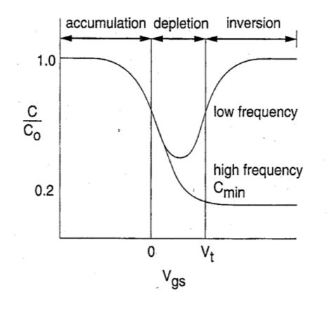
Normalized gate capacitance versus Gate voltage Vgs. High freq behavior is due to the distributed resistance of channel
