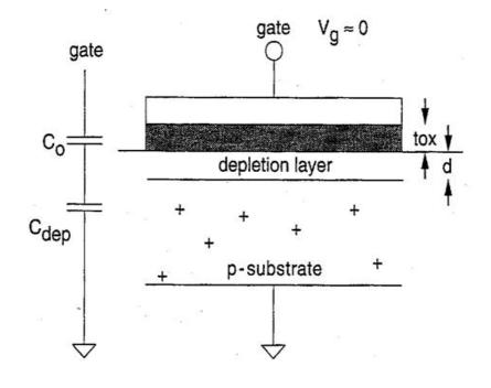
Depletion occurs when Vg is near zero but < Vtn. Here the Cgate is given by CoxA in series with depletion layer capacitance Cdep
