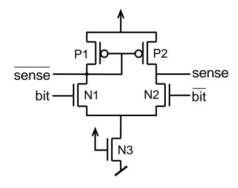
This is a differential analog pair. N3 is a current source where current flows either in left or right branches. Circuit doesn't need a clock but it consumes significant amount of DC power.
