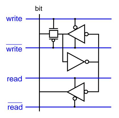
When write=1 the value at the bit is passed to the middle inverter while the upper tri-state inverter is in high Z.
