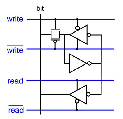
When read=1 the output of the lower tri-state inverter gets connected to the bit so cell's value appears on the bit-line.
