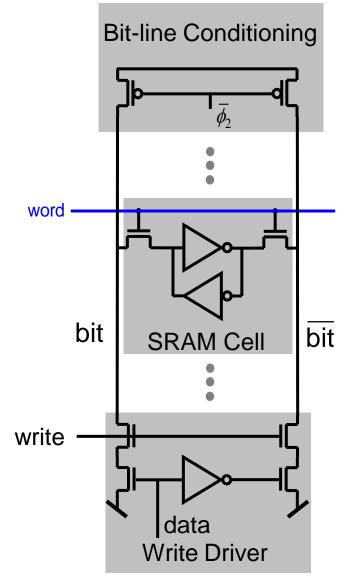
Bit-lines (and complements) are precharged high. At write one is pulled down.
