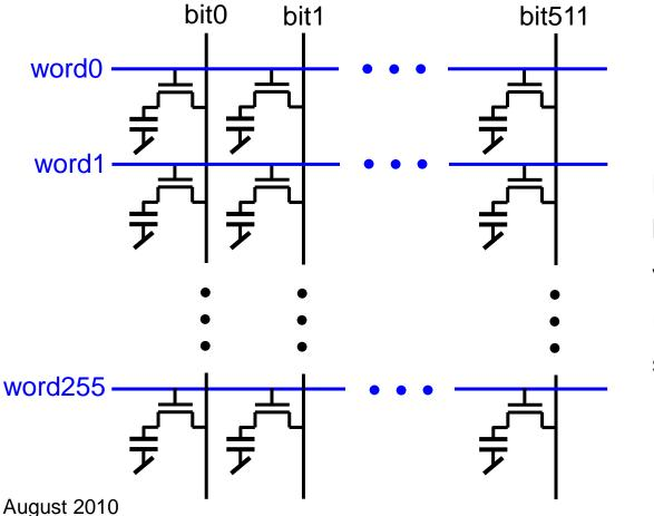
Bit-line capacitance is far larger than cell, hence voltage swing  $\Delta V$  during read is very small and sense amplifier is used.
