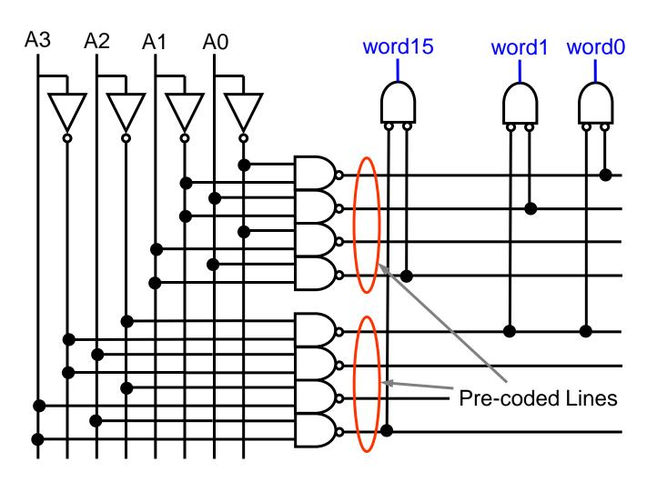
Terms repeat themselves, so pre-decoding will eliminate the redundant ones. This is called *pre-decoding*. Less area with same drive as before.
