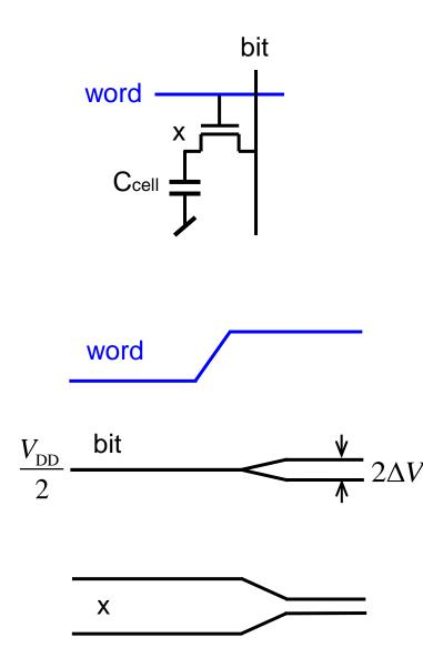
A 1-transistor (1T) DRAM cell consists of a transistor and a capacitor.
