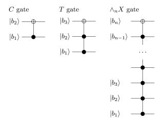
Show (10 points) that the C gate is linear, that is  $C|x \oplus y\rangle = C|x\rangle \oplus C|y\rangle$  where  $x \oplus y$  is the bitwise  $\oplus$ . Suppose U is a quantum circuit on n wires composed exclusively of C gates. Conclude that  $U|x \oplus y\rangle = U|x\rangle \oplus U|y\rangle$  (i.e. U is linear). Note that a correct mathematical proof of this would involve *induction* on the number of C gates composing U but I will accept an intuitive explanation.
