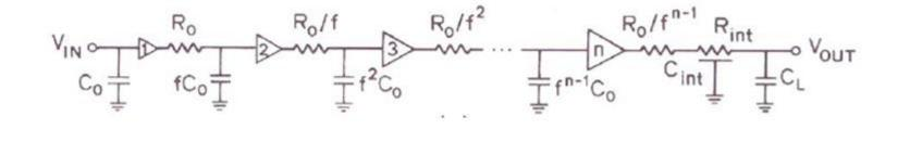
$$T_{50\%} = 0.7(n-1)fR_oC_o + \left(\frac{0.7R_o}{f^{n-1}} + 0.4R_{int}\right)C_{int} + \left(\frac{0.7R_o}{f^{n-1}} + 0.7R_{int}\right)C_L$$
