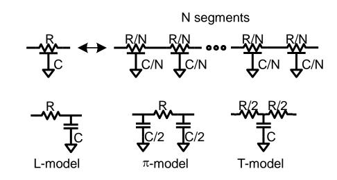
**G** 3-segment  $\pi$ -model is accurate to 3% in simulation
