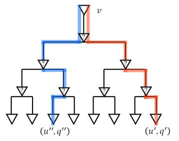
$\max_{\text{buffer insertions}} \left\{ \min_{i} \left\{ q_i - d\left(v, u_i\right) \right\} \right\} \text{ by buffer insertions.}$
