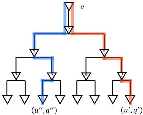
$d(v, u_i)$ : driver to receiver delay. Root required time:  $T = \min_i \{q_i - d(v, u_i)\}$ .
