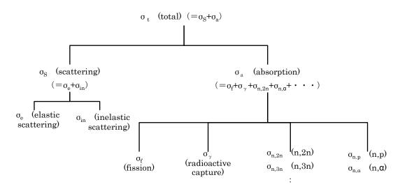
Microscopic cross sections depend on the nucleus, reactions and incident neutron speed (energy)
