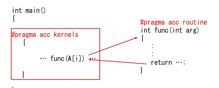
• "routine" directive is required by compiler to generate GPU code
