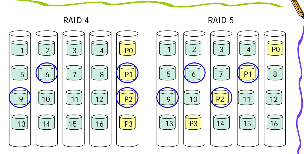
• By distributing parity blocks to all disks, some small writes can be performed in parallel
