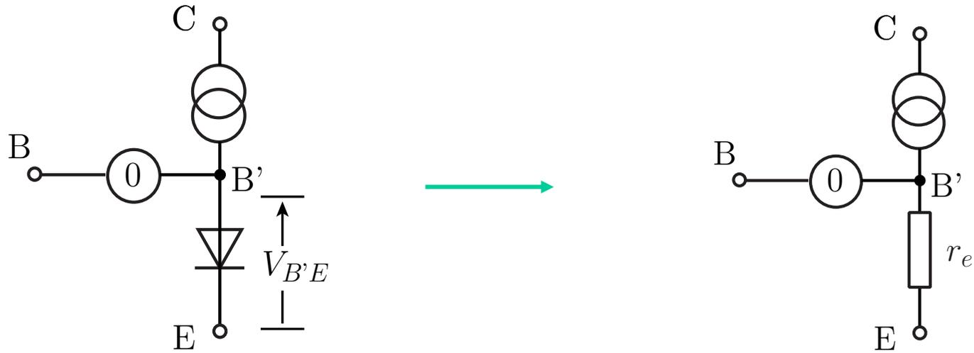
$$r_e = \left[ \frac{\partial I_E}{\partial V_{BE}} \bigg|_{V_{BE} = V_{BEQ}} \right]^{-1} \approx \frac{kT}{qI_{EQ}} = \frac{0.026[\text{V}]}{I_{EQ}[\text{A}]}$$
