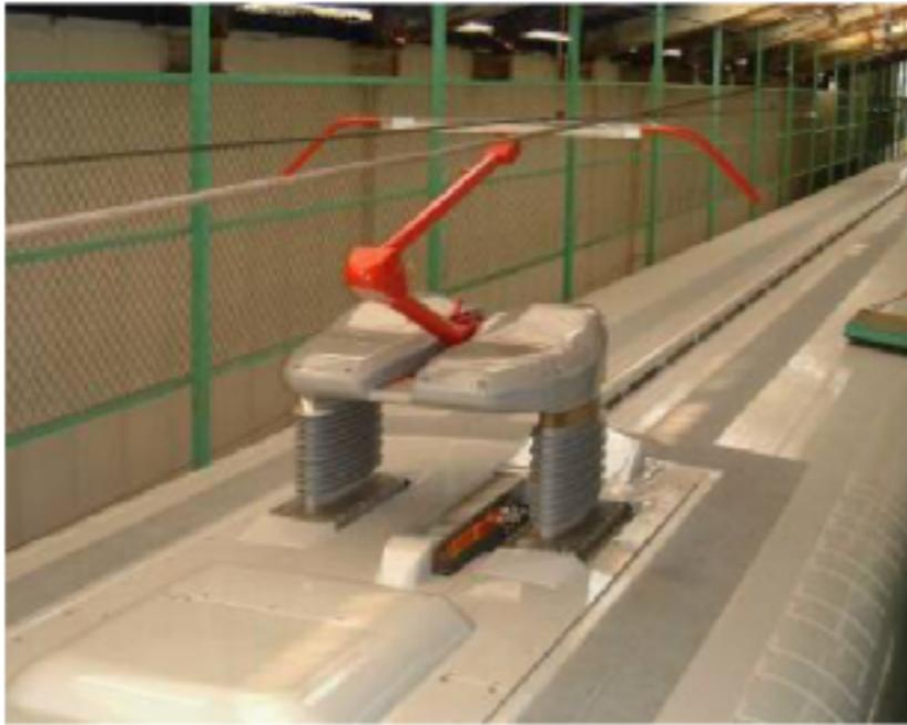
Fig. 2 PS207 type pantograph (series E2)
