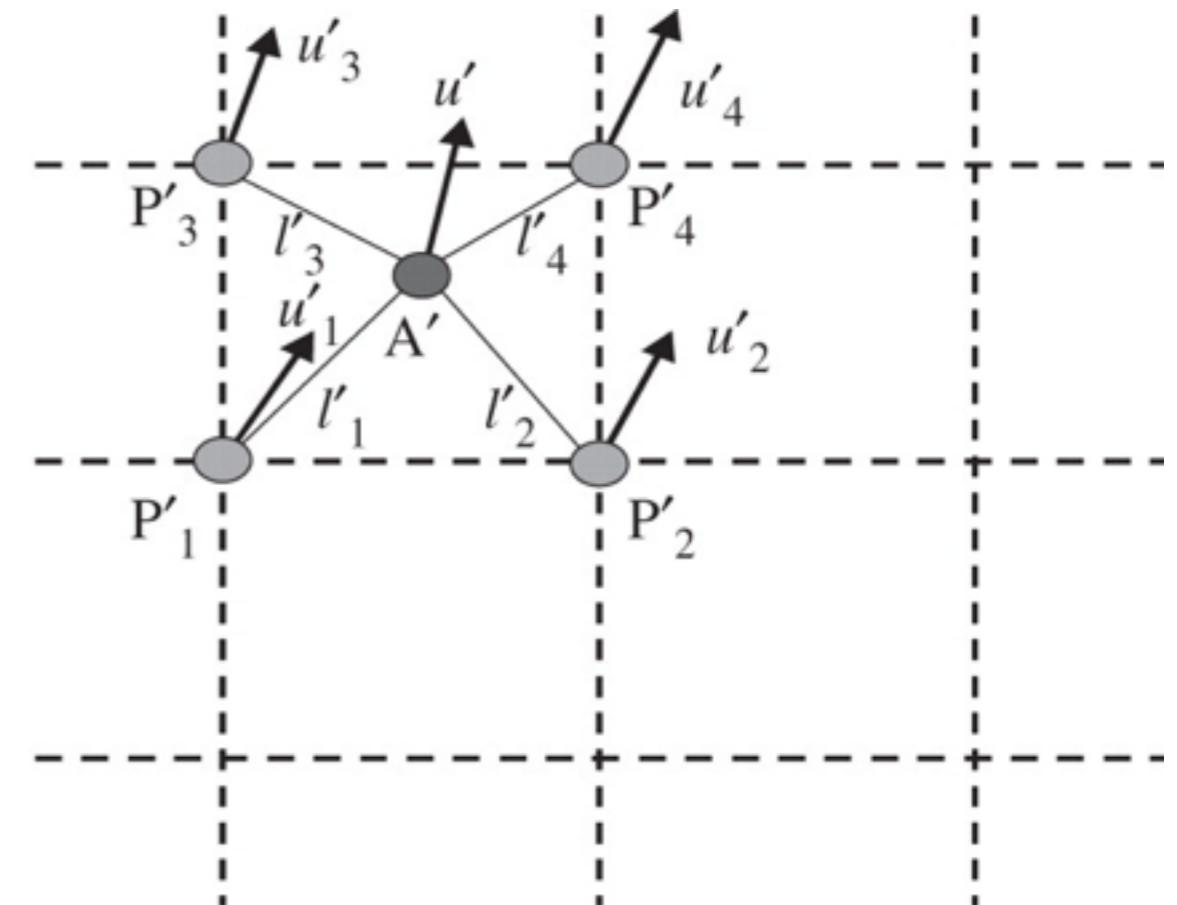
$$u' = \frac{\frac{u'_1}{l'_1} + \frac{u'_2}{l'_2} + \frac{u'_3}{l'_3} + \frac{u'_4}{l'_4}}{\frac{1}{l'_1} + \frac{1}{l'_2} + \frac{1}{l'_3} + \frac{1}{l'_4}}$$
