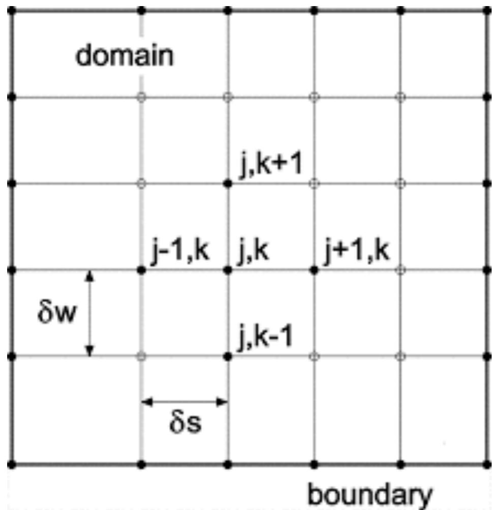
$$\left( \frac{\partial^2}{\partial x^2} + \frac{\partial^2}{\partial y^2} \right) f(x, y) = g(x, y)$$
