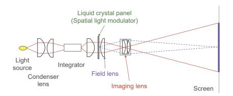
Red: Light flux propagation Blue: Image formation The quality of imaging lens is critical to the projected image quality.
