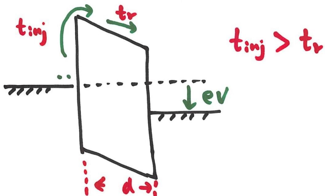
"no accumulation of injected electrons in insulator .."
