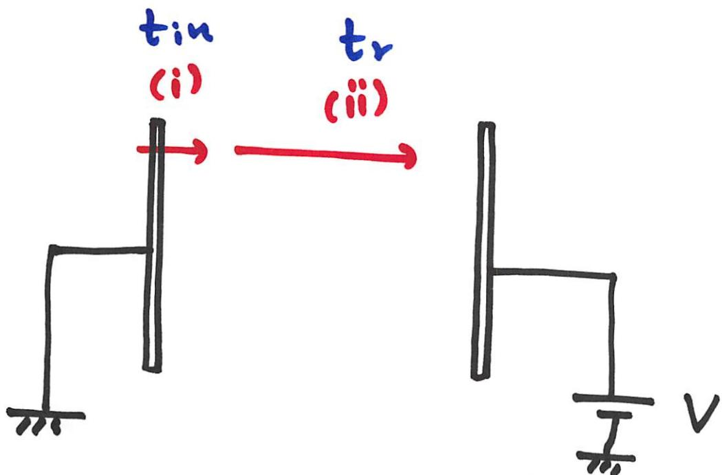
$t_{in} \gg t_r$  injection limited process
