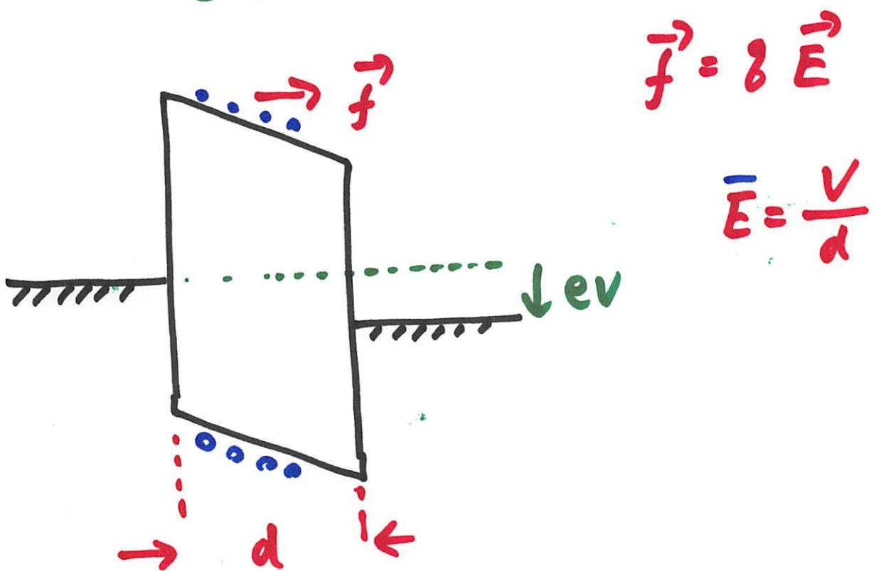
$$I_d \approx e n_0 \mu E = (e n_0 \mu \frac{1}{d}) V \\ = KV$$
