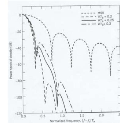
FIGURE Power spectra of MSK and GMSK signals for varying time-bandwidth product.
