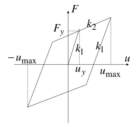
2) What is the equivalent damping ratio if  $k_1 \rightarrow \infty$ 3) What is the equivalent damping ratio if  $k_2=0$
