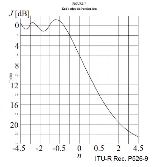
For same *h* (depth of obstruction), *n* is smaller when frequency is lower.
