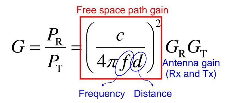
Higher frequency is disadvantageous with respect to coverage.
