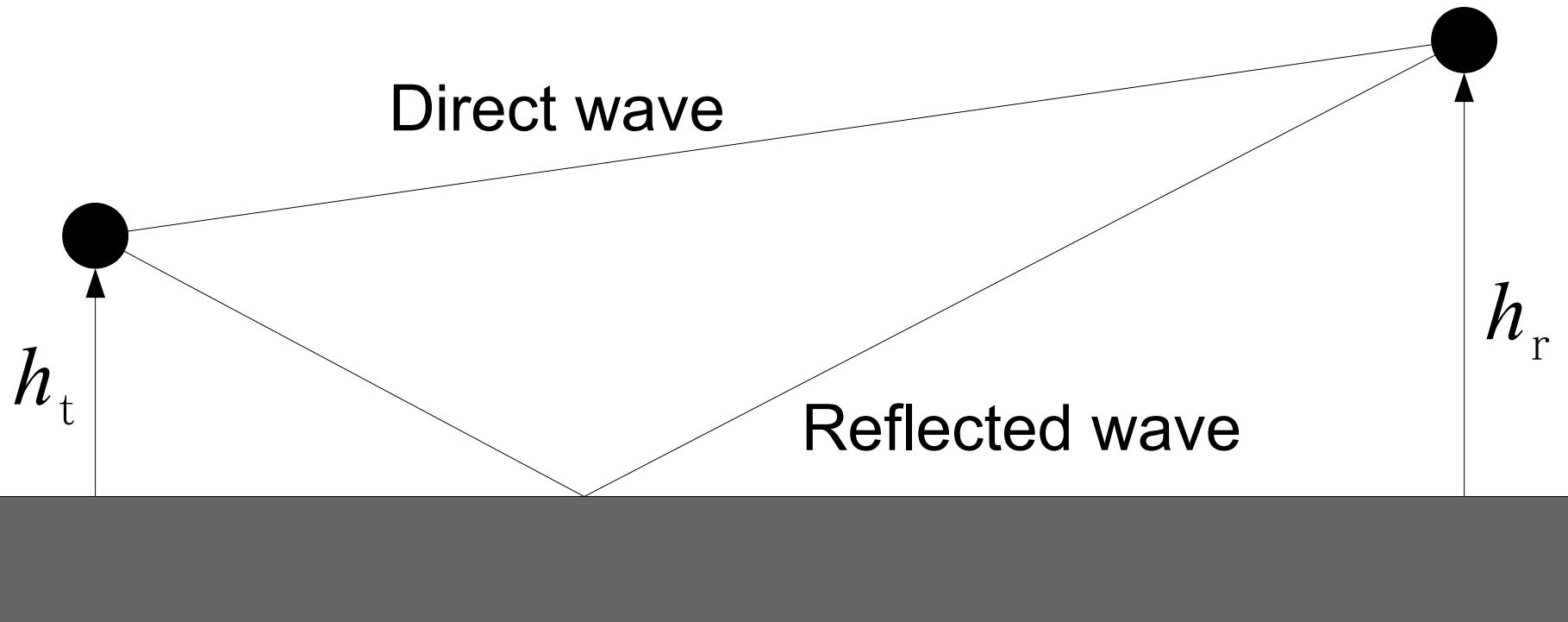
Used for path loss estimation for micro and pico cells 22
