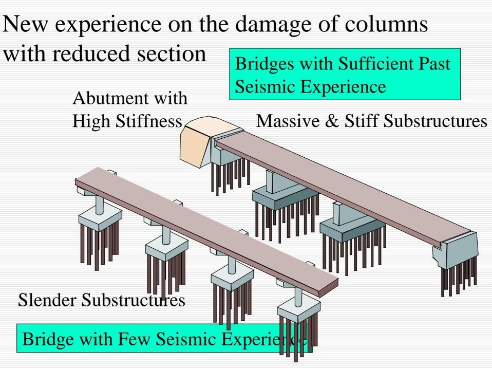
Two Major Factors which Developed The Extensive Damage in Bridges during 1995 Kobe Earthquake
