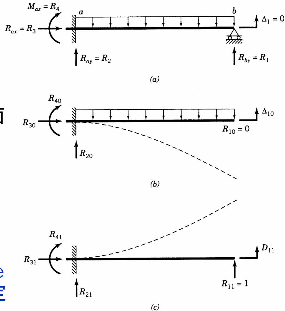
**Figure 10.1** Consistent deformation analysis of a statically indeterminate beam structure. (a) Statically indeterminate structure. (b) Statically determinate primary structure. (c) Unit value of  $R_1$ .
