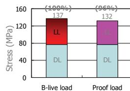
**Stress produced by proof load is almost equal to required stress**
