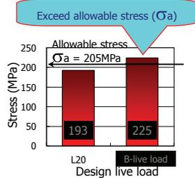
**This bridge should be replaced or strengthened**
