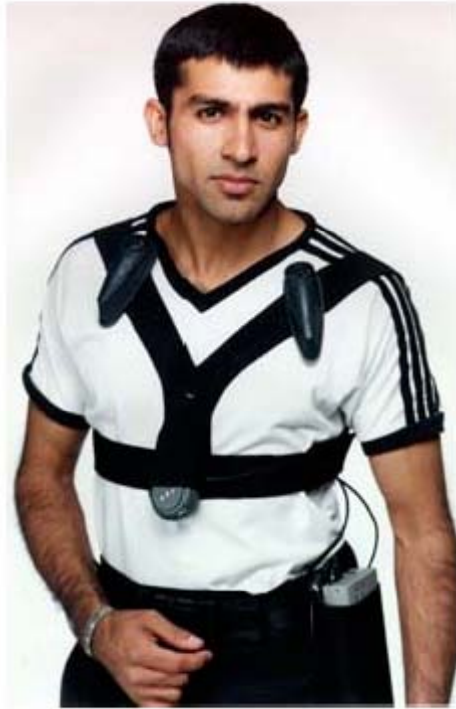
Radio Vest with directional speakers and microphone
