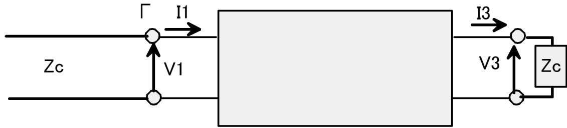
$$\Gamma = \frac{Z_1 - Z_c}{Z_1 + Z_c} = \frac{\frac{A + \frac{B}{Z_c}}{Z_c} - CZ_c - D}{\frac{A + \frac{B}{Z_c}}{Z_c} + CZ_c + D}$$
