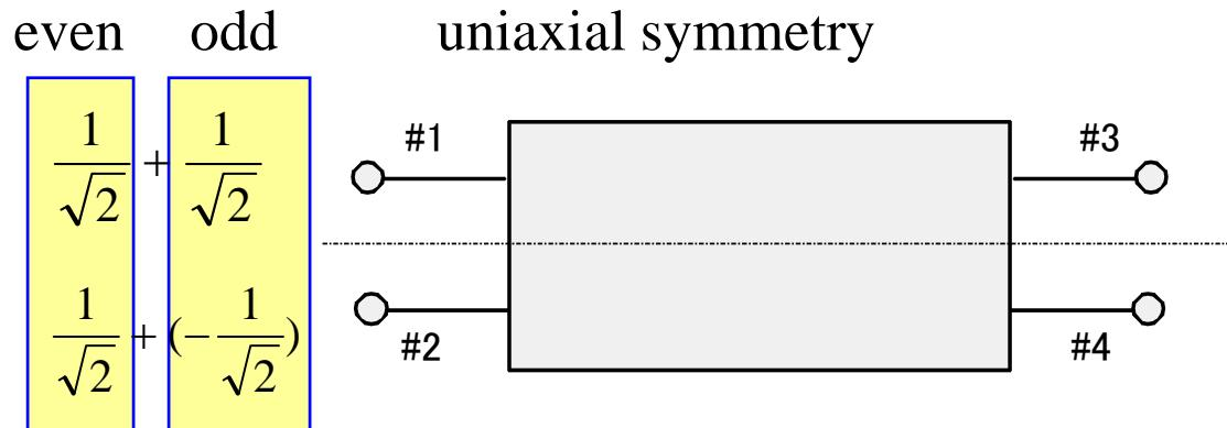
$$\begin{bmatrix} b_1 \\ b_2 \\ b_3 \\ b_4 \end{bmatrix} = \begin{bmatrix} S_{11} & S_{21} & S_{31} & S_{41} \\ S_{21} & S_{11} & S_{41} & S_{31} \\ S_{31} & S_{41} & S_{33} & S_{43} \\ S_{41} & S_{31} & S_{43} & S_{33} \end{bmatrix} \begin{bmatrix} a_1 \\ a_2 \\ a_3 \\ a_4 \end{bmatrix}$$
