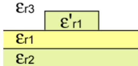
(g) rib (ridge) waveguide
