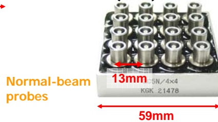
Planar Pitch-Catch Array Probe Miki et al. (2003)
