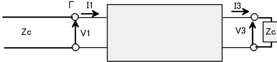
$$\Gamma = \frac{Z_1 - Z_c}{Z_1 + Z_c} = \frac{\frac{B}{Z_c} - CZ_c - D}{\frac{B}{Z_c} + CZ_c + D}$$
