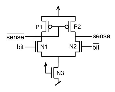
This is a differential analog pair. N3 is a current source where current flows either in left or right branches. Circuit doesn't need a clock but it consumes significant amount of DC power.
