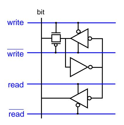
When read=1 the output of the lower tri-state inverter gets connected to the bit so cell's value appears on the bit-line.
