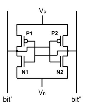
bit' and bit" are initialized to  $V_{DD}/2$ .  $V_p=0$  and  $V_n=V_{DD}/2$ , so all transistors are initially OFF.
