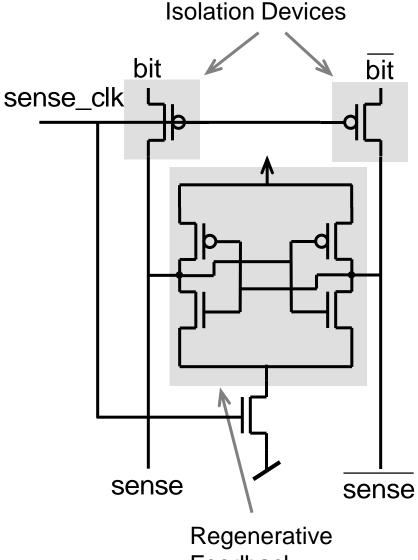
Sense amplifiers are susceptible to differential noise on bit-lines since they respond to small voltage differences.
