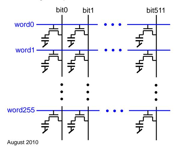
Bit-line capacitance is far larger than cell, hence voltage swing  $\Delta V$  during read is very small and sense amplifier is used.
