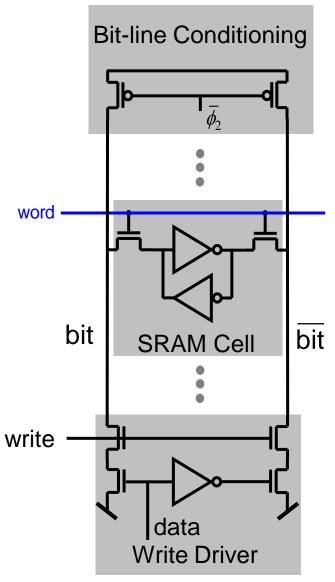
Bit-lines (and complements) are precharged high. At write one is pulled down.
