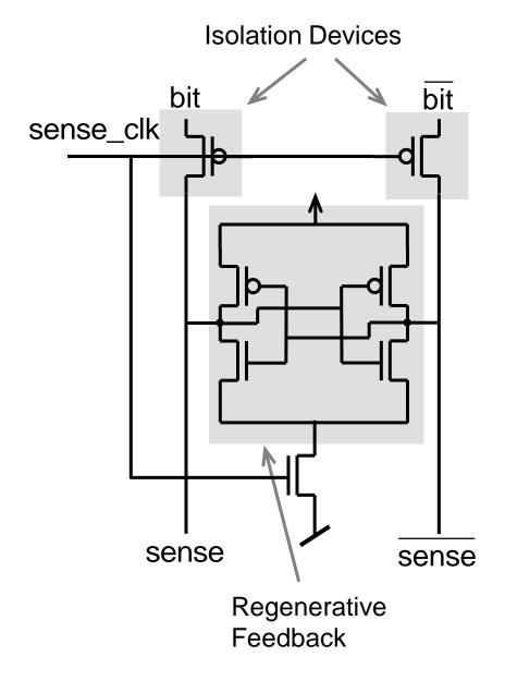
To speed up response bit-lines are disconnected at sensing to avoid their high capacitive load.
