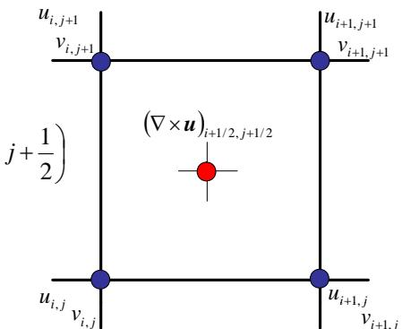
$$\omega_{i+1/2, j+1/2} = \frac{1}{2} \left( \frac{v_{i+1, j+1} - v_{i, j+1}}{\Delta x} + \frac{v_{i+1, j} - v_{i, j}}{\Delta x} \right) - \frac{1}{2} \left( \frac{u_{i+1, j+1} - u_{i+1, j}}{\Delta y} + \frac{u_{i, j+1} - u_{i, j}}{\Delta y} \right)$$
