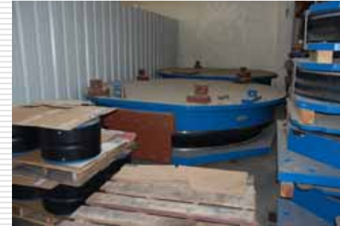
Friction Pendulum System for Carrying Over 10,000 tf Structure
