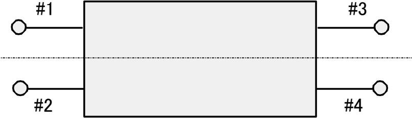
$$\begin{bmatrix} b_1 \\ b_2 \\ b_3 \\ b_4 \end{bmatrix} = \begin{bmatrix} S_{11} & S_{21} & S_{31} & S_{41} \\ S_{21} & S_{11} & S_{41} & S_{31} \\ S_{31} & S_{41} & S_{33} & S_{43} \\ S_{41} & S_{31} & S_{43} & S_{33} \end{bmatrix} \begin{bmatrix} a_1 \\ a_2 \\ a_3 \\ a_4 \end{bmatrix}$$
