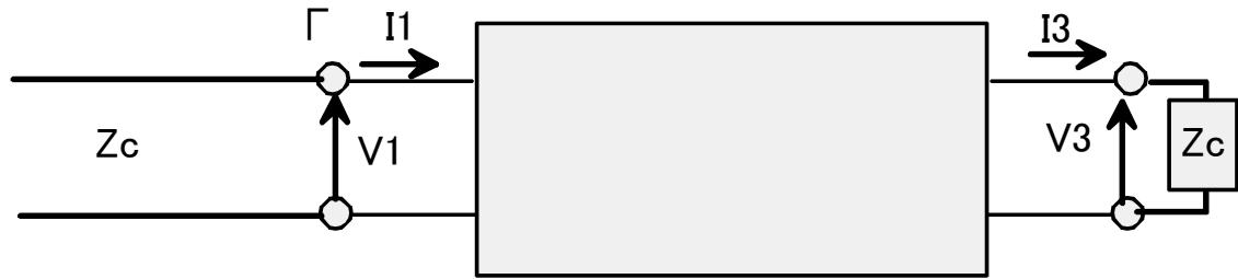
$$\Gamma = \frac{Z_1 - Z_c}{Z_1 + Z_c} = \frac{A + \frac{B}{Z_c} - CZ_c - D}{A + \frac{B}{Z_c} + CZ_c + D}$$
