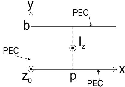
$$E_z = \frac{1}{j\omega\mu} (k^2 - k_z^2) \Psi_{TM} \quad \text{Boundary condition} \quad E_z = 0 \quad (x=0 \quad \text{and} \quad y=0, b)$$
