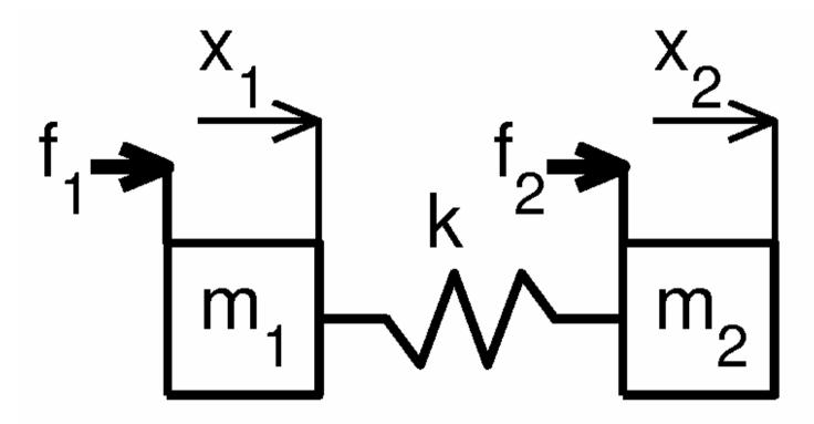
Analytical model of a two-degree-of-freedom mechanism
