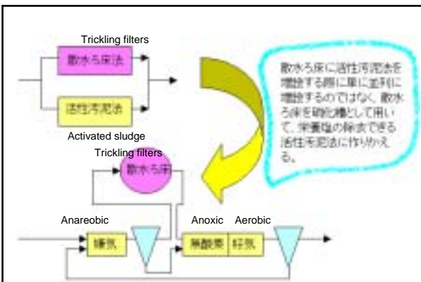
A schematic diagram of the modification of the wastewater treatment plants
