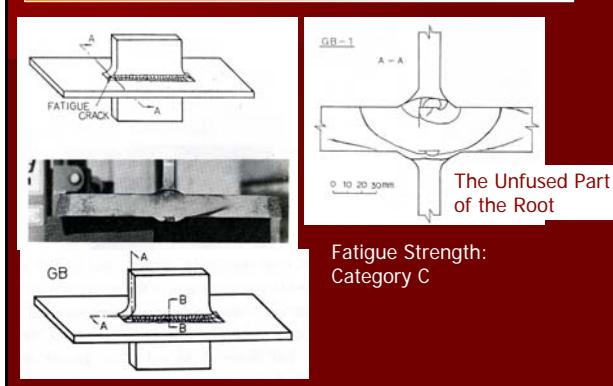
Fatigue Crack in Out-of-Plane Gusset Joints
