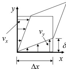
$$\text{変形率} = \frac{\delta}{\Delta x} = \frac{\partial v_y}{\partial x} [\text{s}^{-1}]$$
